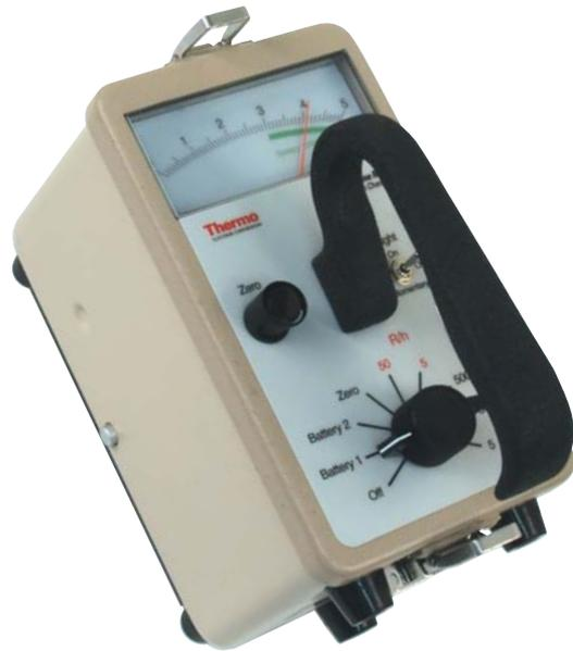
The ionization chamber is vented to atmospheric pressure and is specifically designed to have a flat energy response into the x-ray region. The detector is fully temperature compensated, eliminating any need for temperature correction. Each instrument is factory calibrated to gamma radiation. A single rotary switch turns the instrument off, checks the batteries, checks the zero setting, and selects the range of operation. An ergonomically located switch illuminates the meter. Internal
