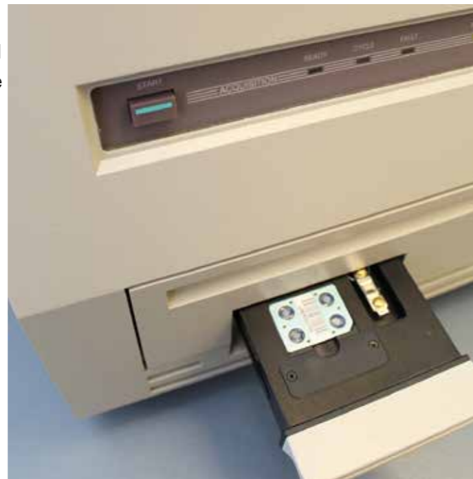
The Harshaw 4500 is equipped with a planchet heating assembly used for unmounted dosimeters and a precisely controlled non-contact nitrogen gas heating system with dual cooled photomultiplier tubes for reading mounted TLD elements in the form of multi-element cards or extremity dosimeters.
