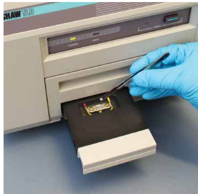
The Harshaw 3500 includes a sample drawer for a single element TLD dosimeter, a linear, programmable and precisely controlled heating system and a cooled photomultiplier tube to measure the TL light output.
