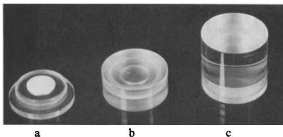
Fig. 1. Perspex dosimeter holders (diameter 20 mm) for patient dose measurements. a) Bottom of a holder containing two LiF-teflon dosimeters. b) Holder used for  $^{60}\text{Co}$  gamma radiation. c) Holder used for 6 and 42 MV roentgen radiation.
